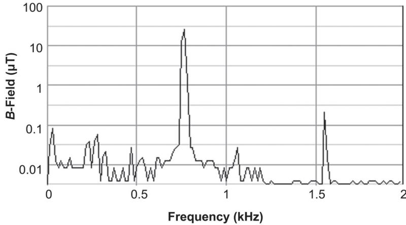
**Figure 7. Spectral analysis of induction heater No. 6.** Notes. Wide band at 30 cm from heater: 28  $\mu\text{T}$ ,  $B$ -field—magnetic flux density.
