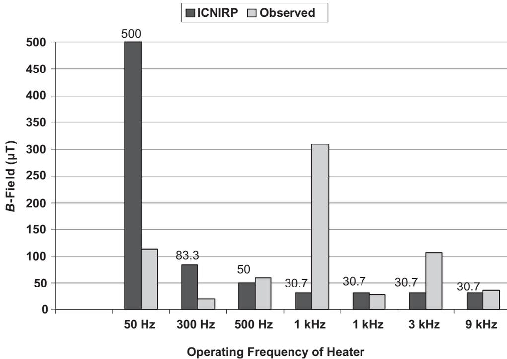
Figure 9. Observed B-field versus the corresponding exposure reference levels of the International Commission on Non-Ionizing Radiation Protection (ICNIRP) [4].
