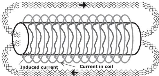
Figure 1. Principle of induction heating.
